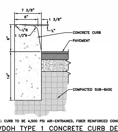
NOTE: CURB TO BE 4,500 PSI AIR-ENTRAINED, FIBER REINFORCED CONCRETE. E WVDOH TYPE 1 CONCRETE CURB DETAIL (CURB1.DWG)
