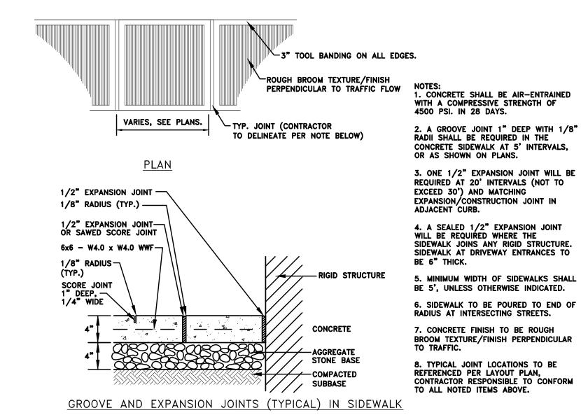
CONCRETE SIDEWALK AT 5' INTERVALS, OR AS SHOWN ON PLANS. 3. ONE 1/2" EXPANSION JOINT WILL BE REQUIRED AT 20' INTERVALS (NOT TO EXCEED 30') AND MATCHING EXPANSION/CONSTRUCTION JOINT IN 4. A SEALED 1/2" EXPANSION JOINT WILL BE REQUIRED WHERE THE SIDEWALK JOINS ANY RIGID STRUCTURE.
