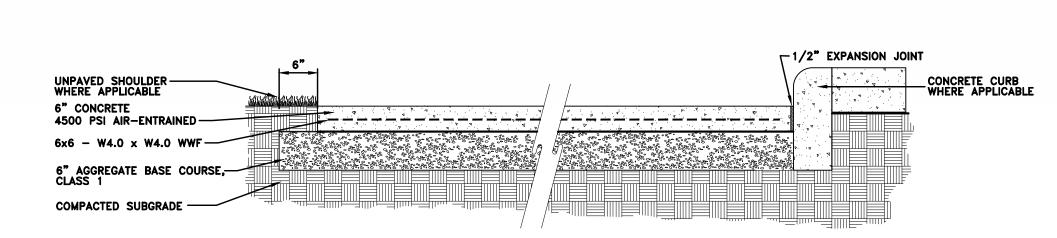
CONCRETE PAVEMENT DETAIL
